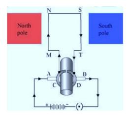
When a current is flowing through the coil MNST, according to Flemings left-hand rule, a downward force acts on the MN side of the coil and at the same time, an upward force acts on ST side of the coil. As a result, the coil rotates anticlockwise.
