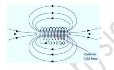
The magnetic field line inside a current-carrying solenoid is parallel. Hence, The magnetic field inside a long, straight, current-carrying solenoid is uniform and same at all points inside the solenoid.
