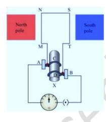
$MNST \rightarrow Rectangular coil$ C and D  $\rightarrow$  Two slip rings A and B  $\rightarrow$  Brushes X  $\rightarrow$  Axle, G  $\rightarrow$  Galvanometer
