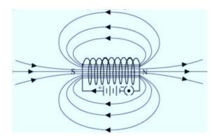
Hence, we can see that when the north pole of a bar magnet is brought near the end connected to the negative terminal of the battery, the solenoid repels the bar magnet. Since like poles repel each other, the right end connected to the negative terminal of the battery behaves as the north pole of the solenoid. Similarly, the other end behaves as a south pole. Therefore it behaves like an electromagnet.
