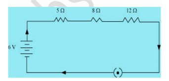
Question 2: Redraw the circuit of question 1, putting in an ammeter to measure the current through the resistors and a voltmeter to measure potential difference across the 12  $\Omega$  resistor. What would be the readings in the ammeter and the voltmeter?
